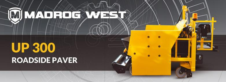
The Roadside paver UP 300 is assigned for paving all kind of bulk materials as well as hot asphalt mass. It is an autonomous machine equipped with an diesel engine and complete hydraulic system. The UP 300 can be installed on any loader of adequate load capacity. The material is transported from the hopper to the road side by conveyor belt.
