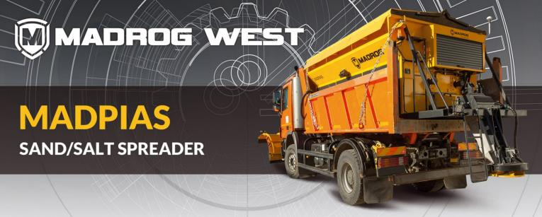
The MADPIAS is the sand/salt spreader for winter road maintenance, designed to meet severe working conditions of the Russian winter. It can be mounted either on the chassis of the vehicle or on the tipper truck. At customer's request our MADPIAS can be equipped with salt moistening system for effective ice removal.
