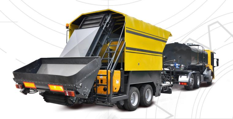
The KOMBAIN is equipped with three pneumatically pressed down rollers which perfectly align the grit on the road surface. The computer control system allows keeping output the both asphalt emulsion and aggregate, exactly to earlier set parameters, even while either machine speed or application width changes. The operator control stand is situated on the front of the KOMBAIN, which helps the operator precisely control the road renovation process.
